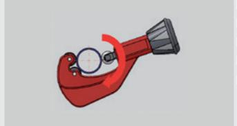
Align the blade with the making of the final dimension of the pipe to be cut, using circular movements.
