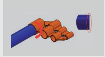
Insert the pipe until it reaches the internal stop of the tool and perform the chamber, using circular moviments.
