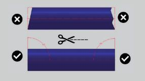
If any pipe needs to be cut, this operation must have a finish free of burrs and sharp edges to avoid
