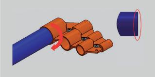
Insert the pipe until it reaches the internal stop of the tool and perform the chamber, using circular moviments.
