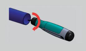
Position the tool and perform deburring, using circular movements.
