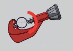
Align the blade with the making of the final dimension of the pipe to be cut, using circular movements.
