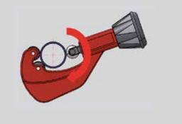
Align the blade with the making of the final dimension of the pipe to be cut, using circular movements.
