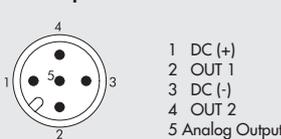
**ANALOG PRESSURE SWITCH WIRING DIAGRAM**
