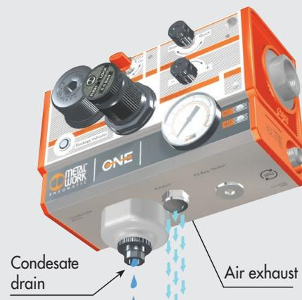
The air in the circuit is relieved via one outlet situated below the unit and fitted with silencer. If you want to convey air relief to prevent the emission of polluted air into the atmosphere, you can replace the silencer and install a fitting. (a pipe with a diameter of at least 6 mm is recommended)
