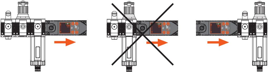
The Syntesi® components can be easily mounted on the outlet side of the FLUX.
